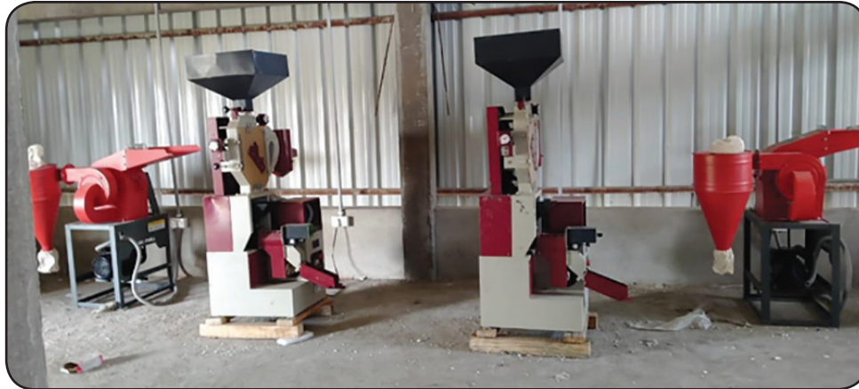
Fig: Inside the Dighalbori CFC – 1 solar rice huller, 1 solar oil extractor, 1 ginger powder machine
